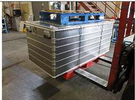
Bottom lift test entry on rear face
