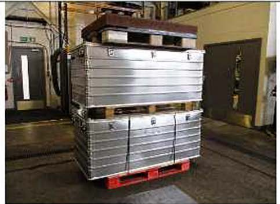
Stack test in progress
