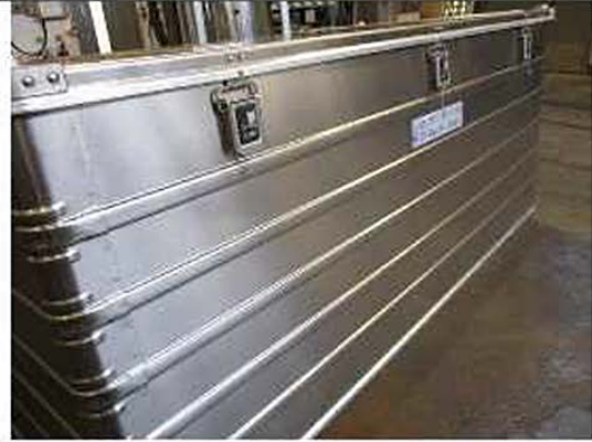
Spot welded seams on sidewall
