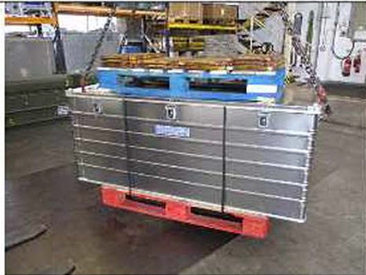
Top lift test in progress
