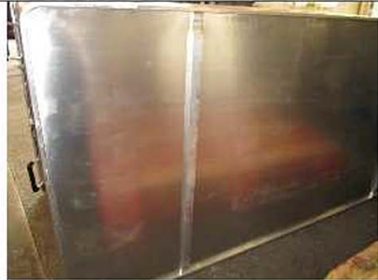
Base view showing panel stiffener
