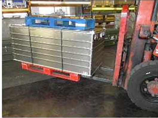
Bottom lift test entry on end face
