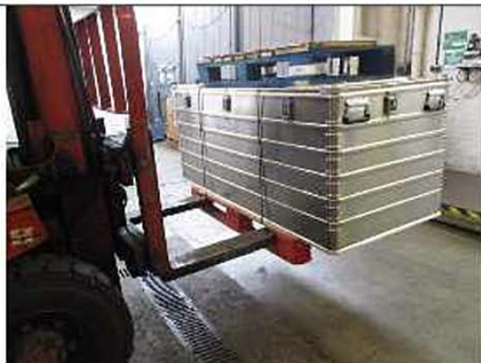
Bottom lift test entry on front face
