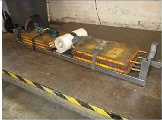
Framework loaded with weights
