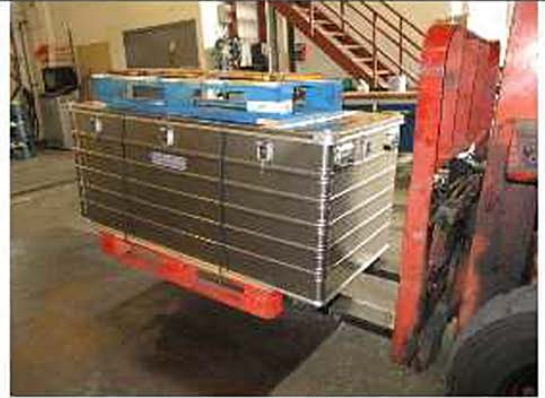
Bottom lift test entry on opposite end face
