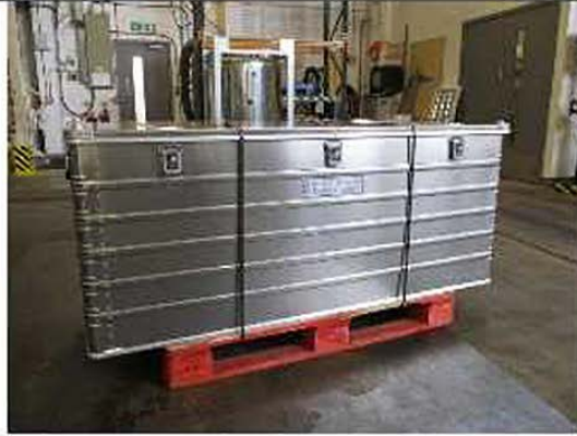
Aluminium large packaging fitted with wooden pallet base submitted for performance testing
